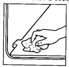
5. After the oven is cool, wipe off any residue or ash with a damp cloth or sponge. If needed, touch up spots with a mild abrasive cleanser or cleaning sponge.
